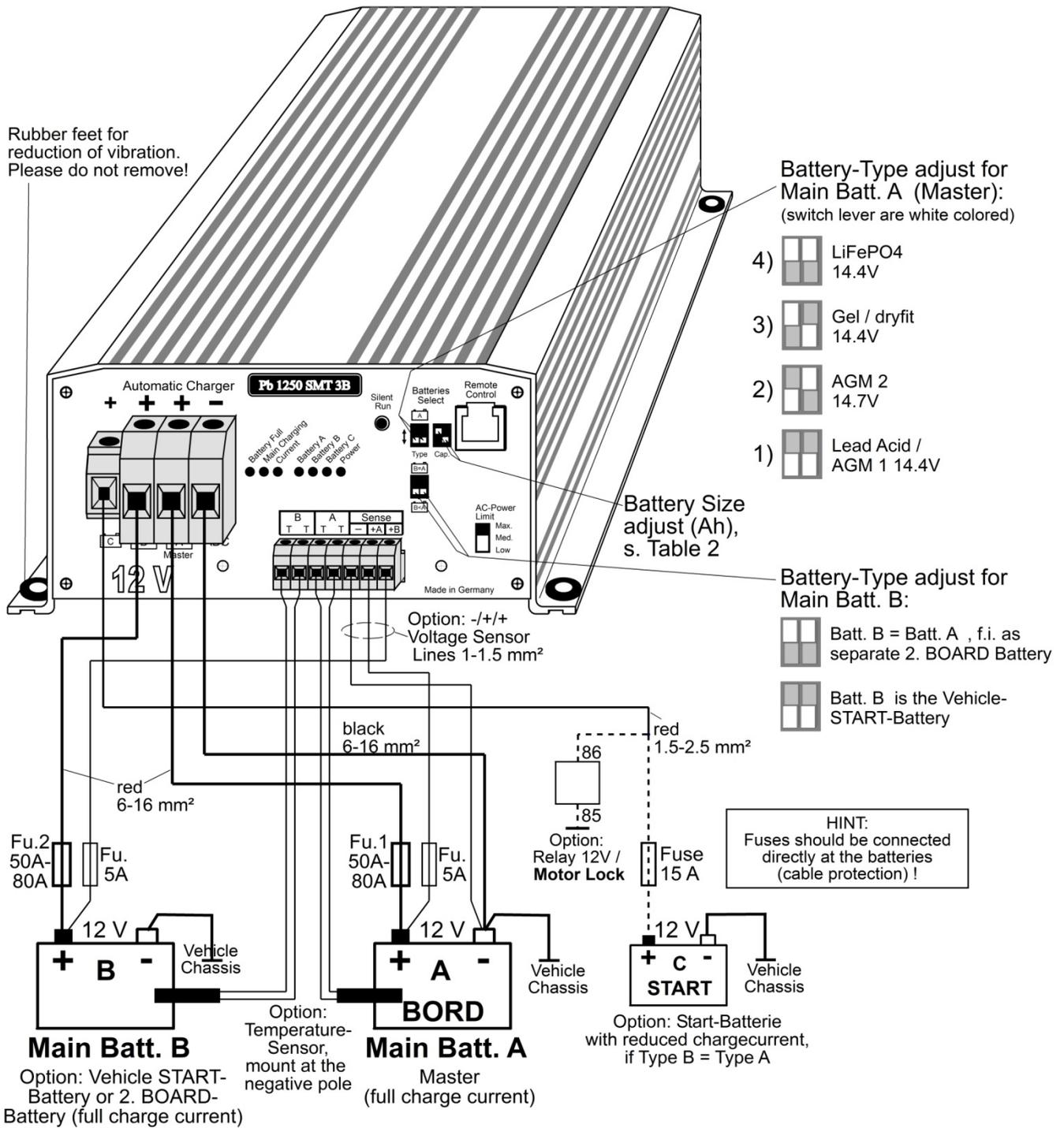
Note: For safety reasons, the unit does not operate with LiFePO4 batteries, **unless** the temperature sensor "A" had been connected (temperature sensor 825, order No. 2001, is required)! The sensor must be screwed-down to the negative pole of the battery. Recommended also for lead batteries, if the battery is exposed to strong variations in temperature!
